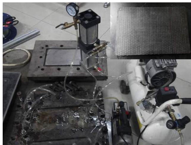
Fig. 2. Photograph illustrating the infiltration of the carbon nanotube/carbon fiber preforms with vacuum-assisted resin transfer molding (VARTM).
